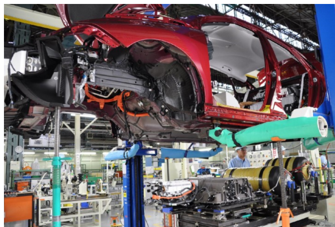
Fig. 2 – installation of the fuel cell stack in the Mirai vehicle at Motomachi plant.
