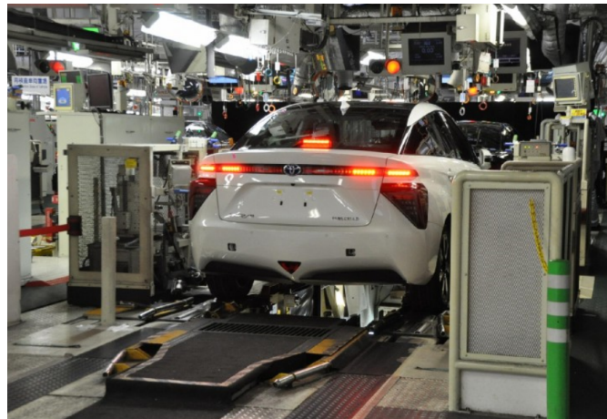
Fig. 3 – Final inspection of the Mirai at Motomachi plant.
